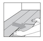
The released plank can then be pulled out. However, never bend installed planks backwards, as this will damage the planks.
